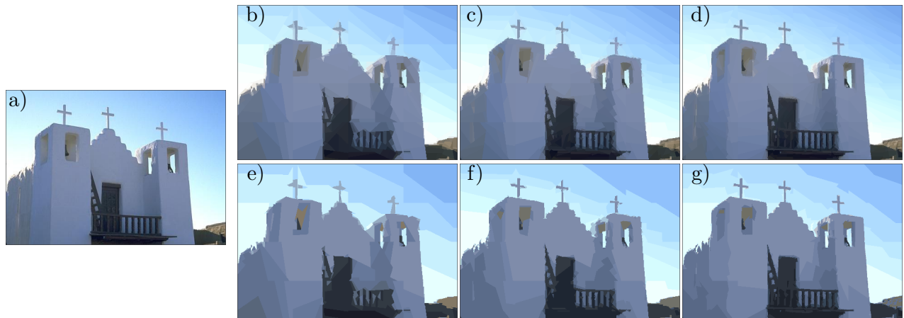
Fig. 2. Split and merge segmentation of colored image: a) original image with 481 \times 321 pixels; b)c)d) Wedgelet approximation with 200, 500 and 1000 graph wedgelets; e)f)g) Segmentation of image by merging the decompositions in b)c)d), respectively.
